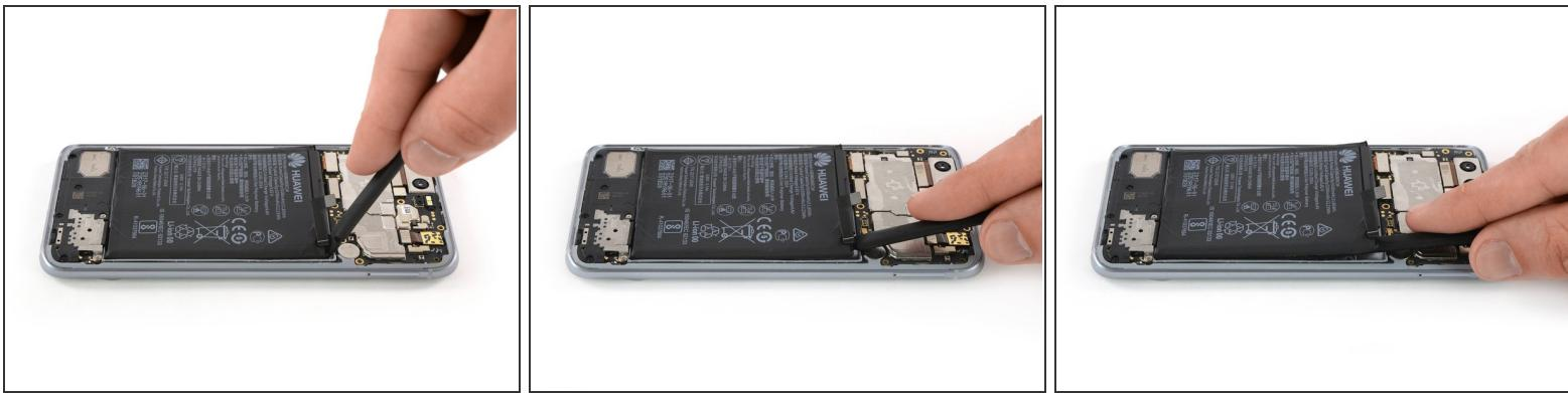
**⚠** Try your best not to deform the battery during the following removal process. Soft-shell lithium-ion batteries can leak dangerous chemicals, catch fire, or even explode if damaged. Do not use excessive force or pry at the battery with metal tools.
