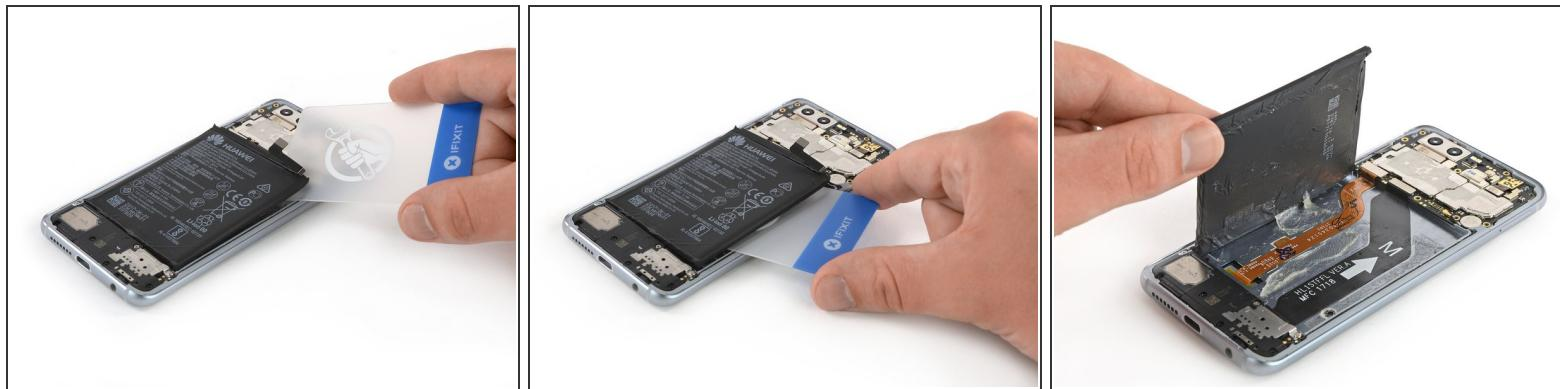
**⚠** The display and interconnect flex cables are running underneath the battery. Don't damage them while cutting the remaining adhesive.
